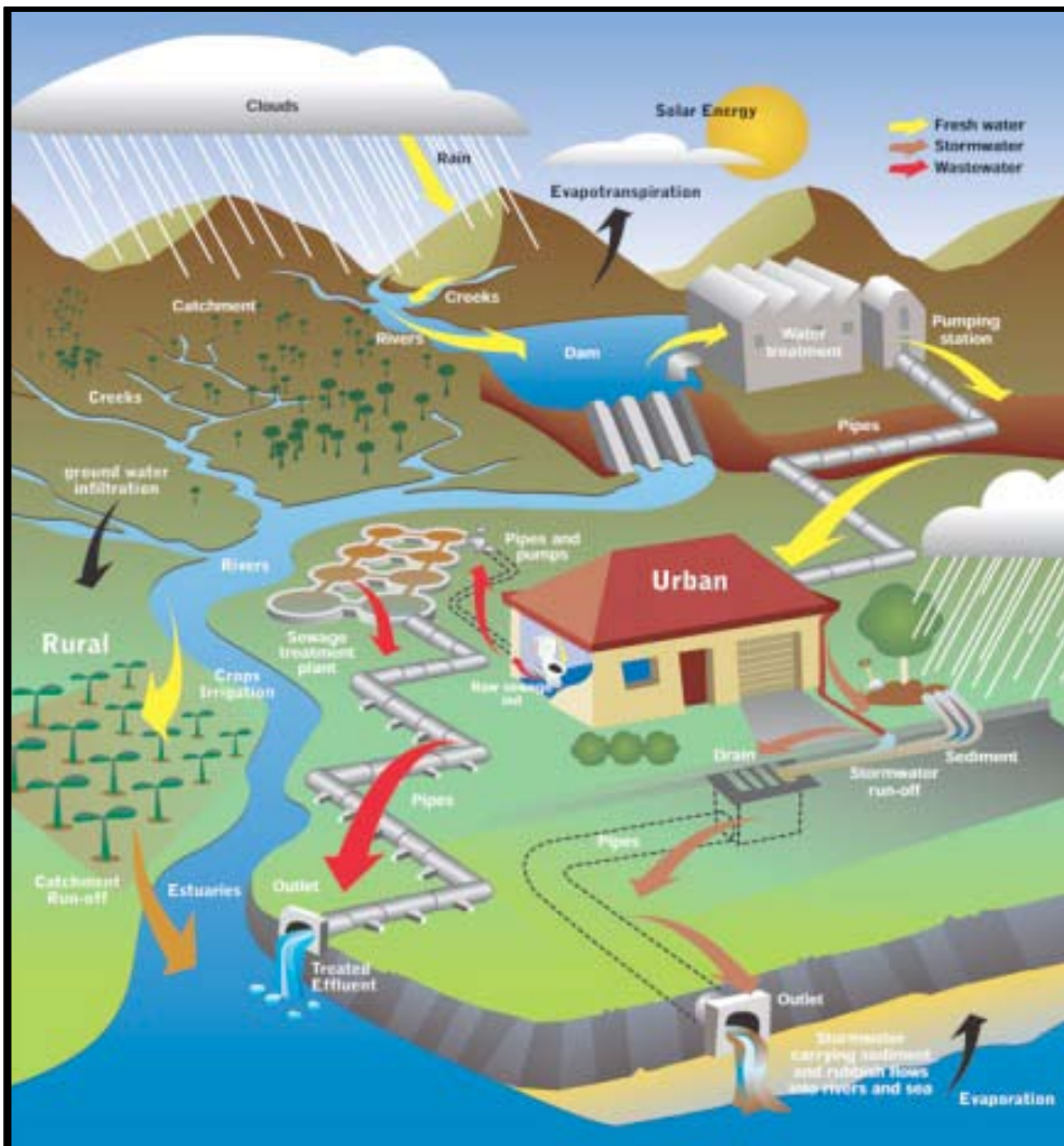
This graphic represents nature's hydrologic cycle, which describes the continuous flow of water on, above, or below the earth.
